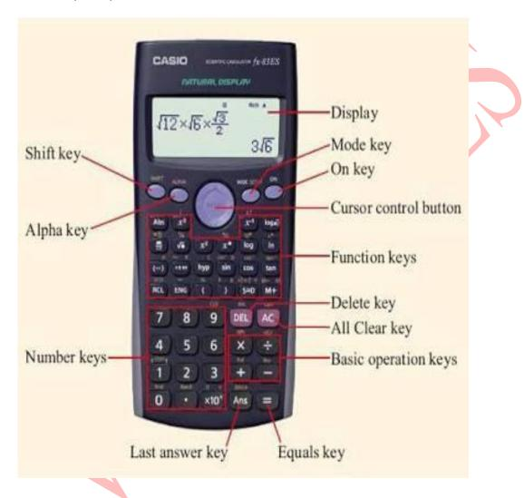
Components: In general, a basic electronic calculator consists of the following component:
